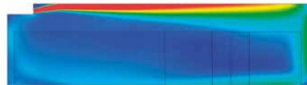
Cut plot 0,1 m ≈ 0,33 ft above the floor – air velocity (displayed interval 0 - 0,2 m / s; 0-39,4 ft / min).
