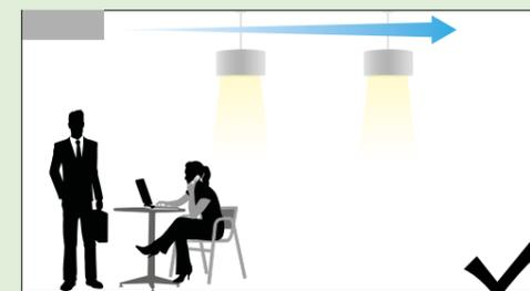
To achieve the most efficient supply conditions, objects, such as light fittings installed directly in the ceiling, should be avoided. Light fittings should be lowered so that the inlet has free access to the room.
