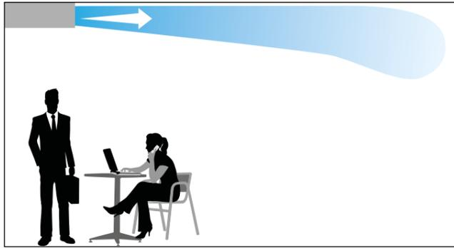
The ceiling-mounted units all ventilate using the mixing principle where fresh air is supplied into the room near the ceiling using the Coanda effect.
